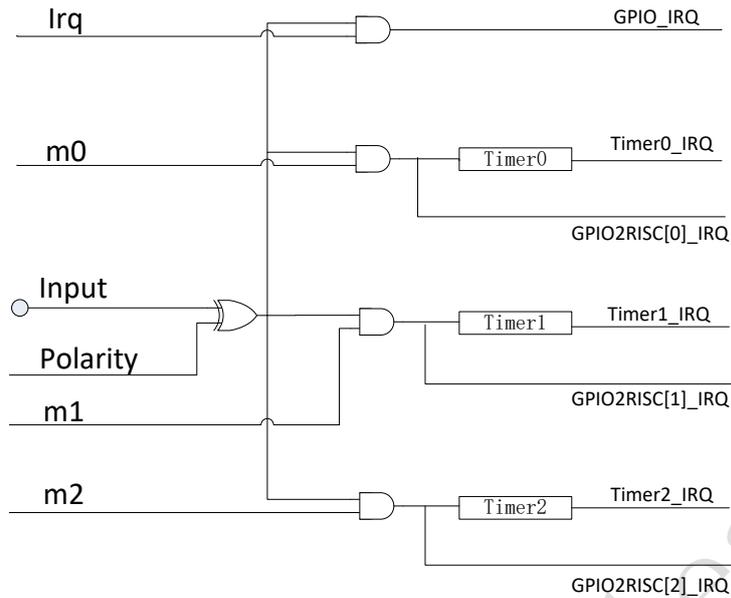
Figure 7- 1 Logic relationship between GPIO and related modules
