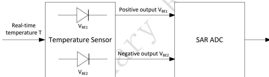
Figure 12- 1 Block diagram of temperature sensor
