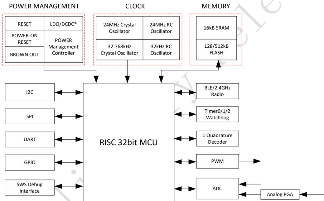
Figure 1- 1 Block diagram of the system
