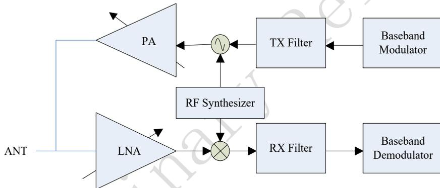
Figure 3- 1 Block diagram of RF transceiver
