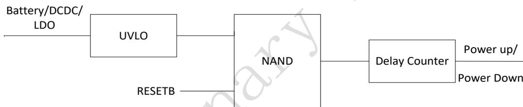
Figure 2- 3 Block diagram for power up/down
