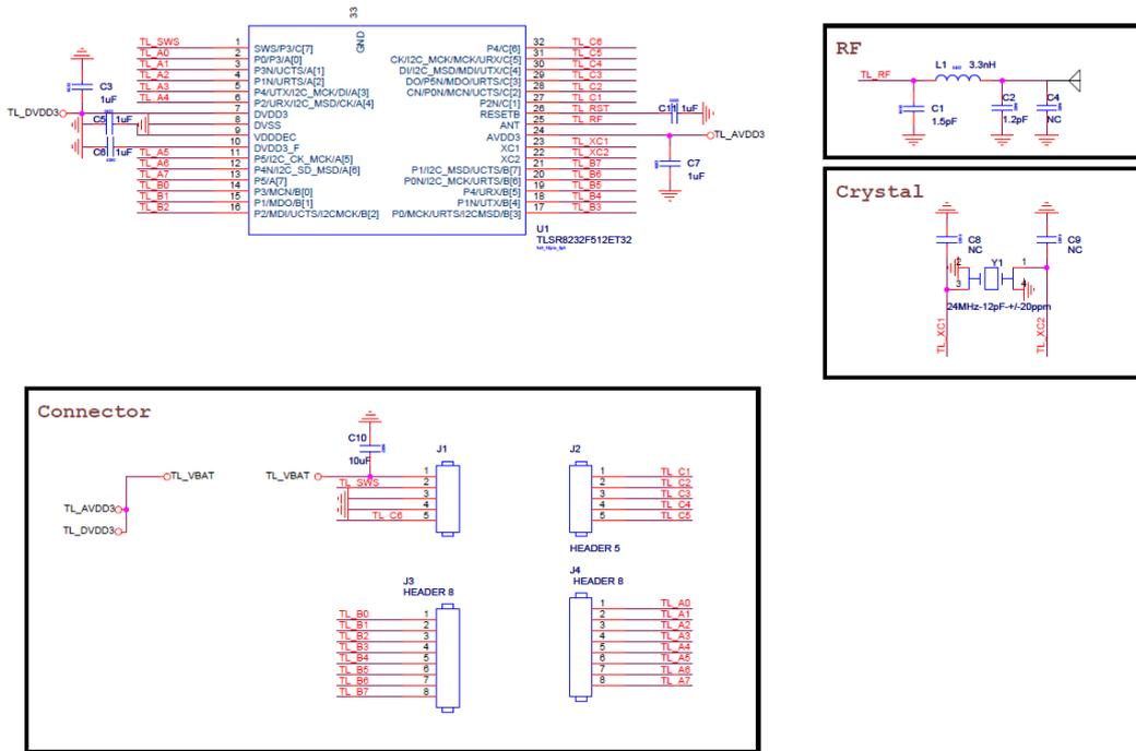
Figure 15-1 Reference Schematic
